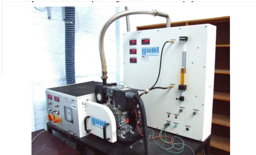
Fig. 8 An engine test lab system with a drive motor and dynamometer produced by GUNT (2010)
