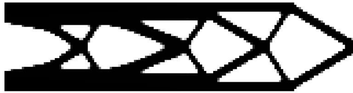
Figure 8: QSOF (solution if using 10^{-8} as convergence criteria at iteration 50 C_{50}=182.6 Nmm) V_0=0.55 ; ER=1.5\% ; H_s=0.5 ; H_d=0,5 (it.<50); \beta=4,6,8\dots
