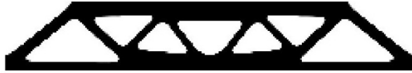
Figure 12. Solution obtained with QSQF ( C_{200}=2.41 Nmm; j_1\%=93 , pcw.) for Problem 2 V_0=0,7 ; ER=5\% ; H_s=0,5 ; H_d=0,2 (it.<30); \beta=5,6\dots
