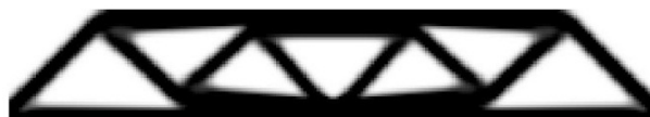
Figure 10: Solution obtained with SIMP& OC ( C_{200}=2.551 Nmm; j_{1\%}=30 ) for Problem 2 r_{\min}=3.0 mm
