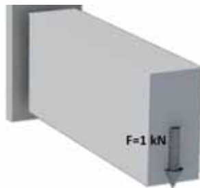
Figure 13: Boundary conditions for Problem 3
