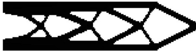
Figure 6d: Solution obtained with QSQF ( C_{200}=184 Nmm; j_{1\%}=52 , inv.pow) for Problem 1 V_0=0.7 ; ER=1.5\% ; H_s=0.5 ; H_d=0,4 (it.<40); \beta=4,5,6\dots
